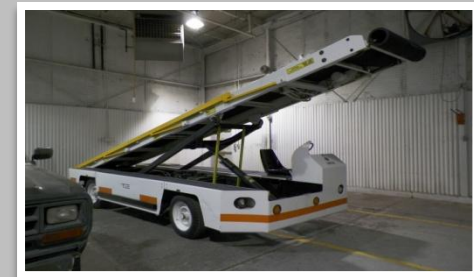
S&S Tug Mobile Belt Loader 11' Height Range
