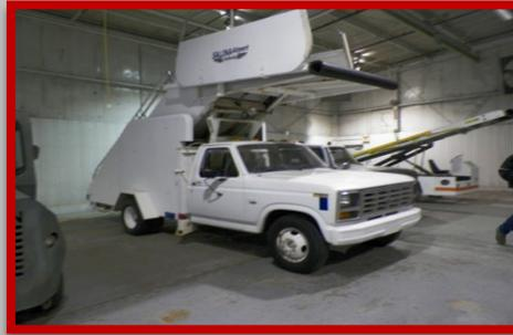
**PS4: Self Propelled Passenger Air Stair**
