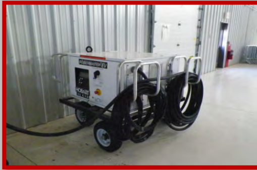
Hobart AC Ground Power Unit 400 Hz Solid State 460 VAC 50-60Hz
