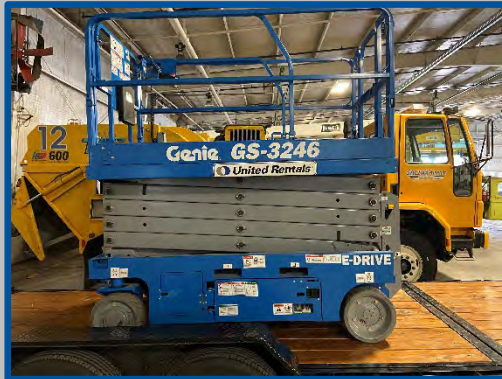
Scissor Lift 38 ft. Working Height Max. 32 ft. Platform Height
