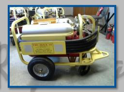
**Description**: Hobart AC Ground Power Unit 28 VDC Solid State, 3ph/208-230-460V/60Hz
