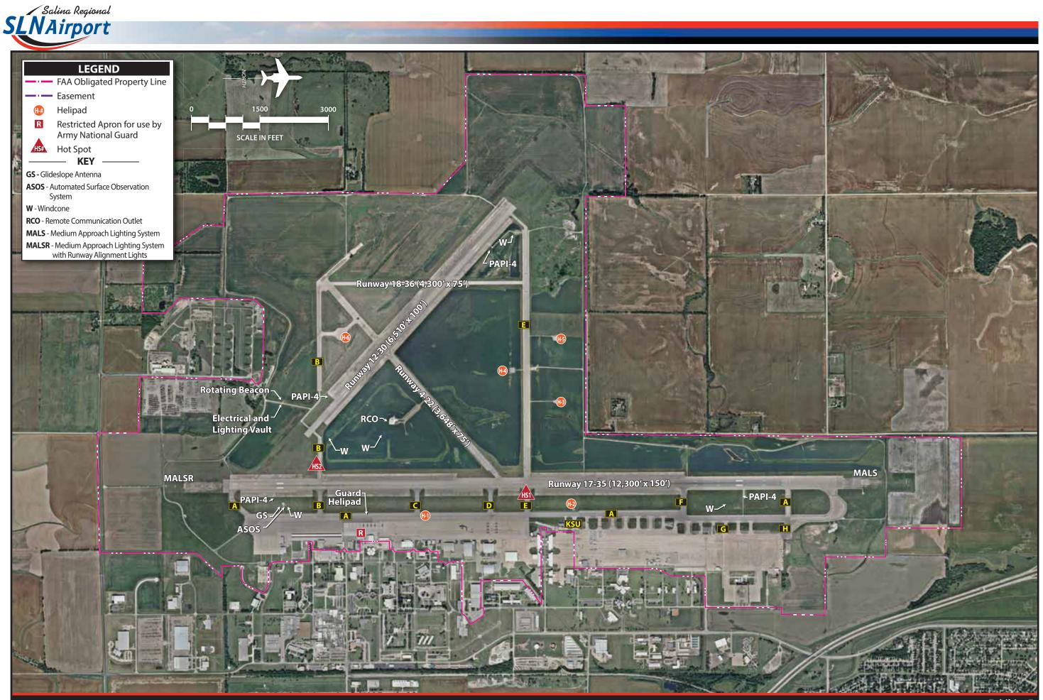
Exhibit 1F Exisiting Airside Facilities taxiways simply connect the two runway ends with the parallel taxiway. The northern entrance/exit Taxiway A is aligned at a 90 degree angle interface with Runway 17 and Taxiway A. The southern entrance/exit Taxiway A is aligned with Runway 35 in an angular fashion sometimes referred to as a spiral exit.
